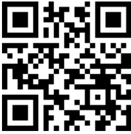
Figure 3-5. QR Code for the string “Hello world qrcode.” The image should appear identical when produced by any of the libraries.
